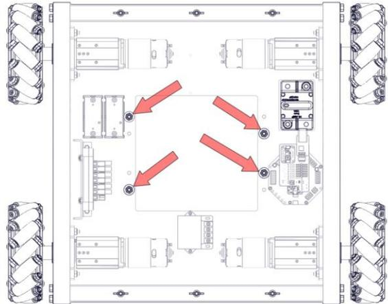
**Step 11:** When taking the battery in and out of the Rover, use (4) 10-32 wingnuts (am-1483) placed on the standoffs created in step 10 to hold down the (2) battery straps (am-2940) as shown.
