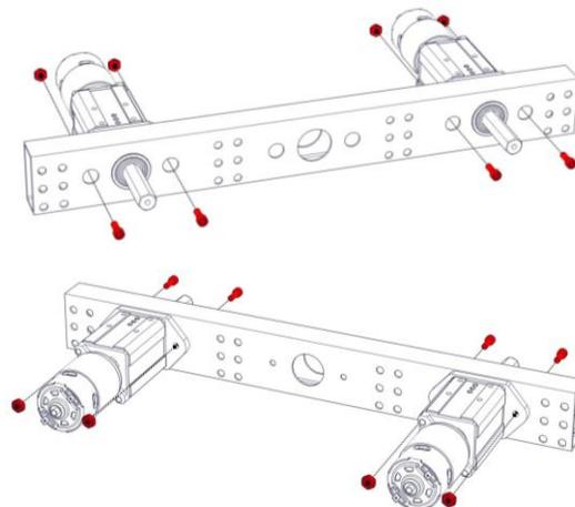
**Step 3:** Using twelve (12) ¼-20 x 1.75 inch Self-Tapping Screws (am-1372), join the Rover Drive Rail Assembly from Step 2 to two Rover End Rails (am-4131). The Rover End Rails will have the rounded face towards the bottom to ensure the top and bottom faces of all three rails are flush. Use eight (8) 0.375 inch OD x 0.875 inch long Aluminum Spacers (am-1513) inside the Rover Side Rail with the screws that are not adjacent to the bottom wall to prevent crushing the tube.
