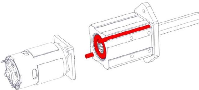
**Step 8:** Attach the Redline Motor with 16 Tooth Pinion (am-3775a\_16t) to the 57 Sport Back Plate (am-3765) using M4 x 8mm screws and lock washers included with the motor.
