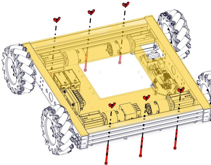
**Step 10:** Run (4) 3.5IN 10-32 socket head cap screws through the center of the rover in the pattern shown. Place (8) 1IN 10-32 spacers between the top and bottom plates along the screws. Above the top plate, put (1) 0.5IN spacer on each screw and hold the assemblies together with (1) 10-32 nylock nut each.
