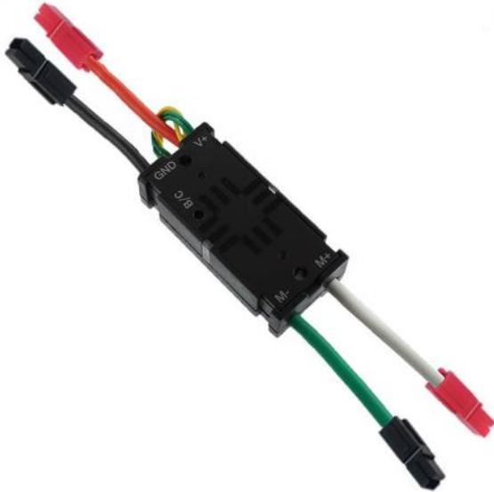
**Step 5:** Add four (4) Victor SPX Speed Controllers (am-3748) in two stacks of two with the CAN wires oriented facing towards the CAN Connector. Use four (4) M4x50 Socket Head Cap Screws (am-1401) and M4 Nylock Nuts (am-1435) to secure the controllers to the top of the Bottom Plate.
