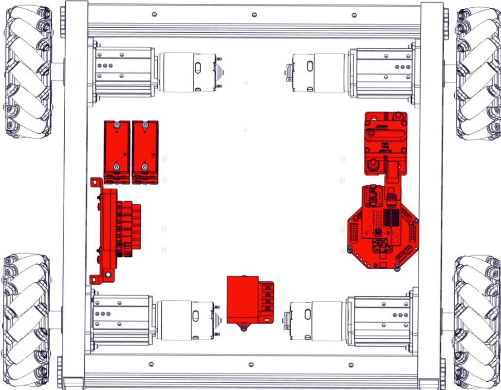
**Step 2:** Mount the PowerPole Distribution Board (am-3699) to the S3 Battery Mount (am-3687) using the 6-32 Socket Head Cap Screws and 6-32 Nylock Nuts included with the Distribution Board Kit, as shown below.
