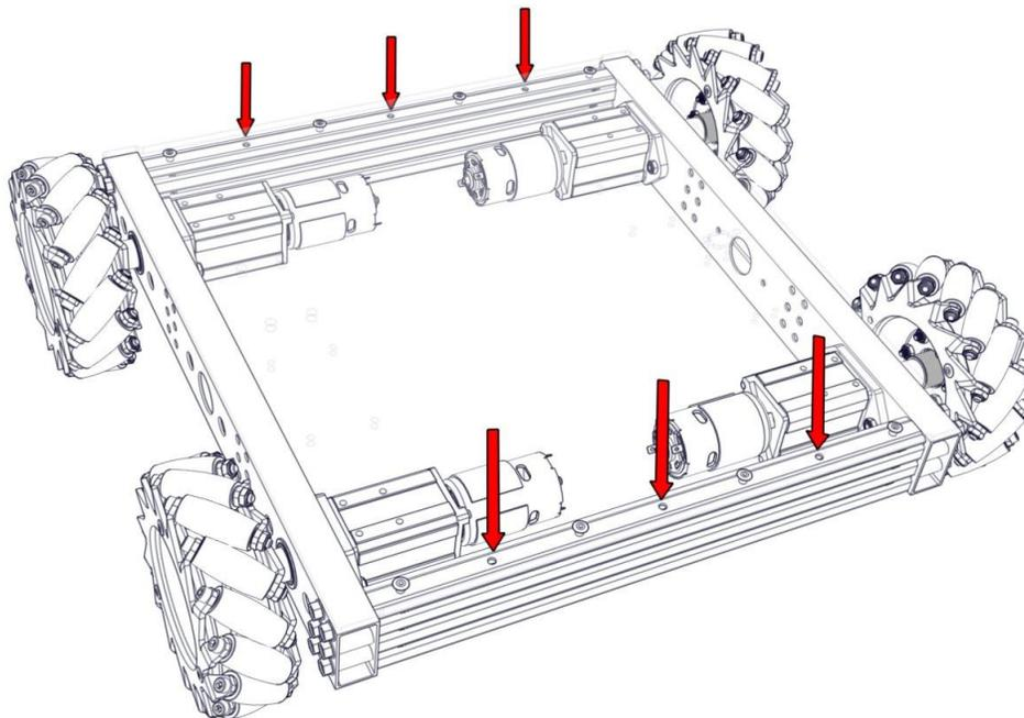
**Step 10:** Flip your chassis over and you have completed the assembly of the Rover 6" Mecanum Chassis. Electronics will be added in the following section. You may skip to **Step 19** of the Electronics Assembly when assembling only the mechanical portion of the chassis or using a custom electronics package.
