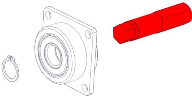
**Step 5:** Replace the snap ring on the new shaft. Be careful to not permanently deform the snap ring by opening it too wide. It should snap into the groove on the output shaft around the full circumference.
