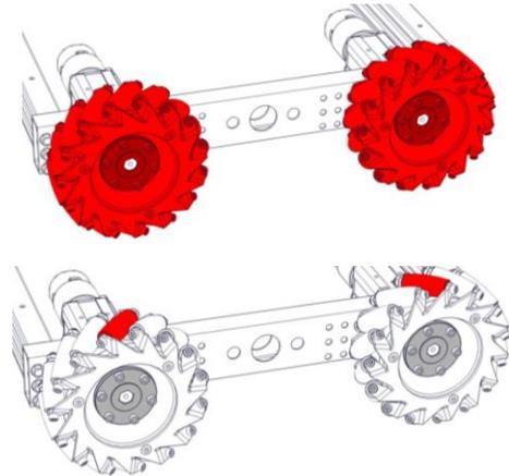
**Step 6:** Capture the wheels on the gearbox output shafts with a #10-32 x 0.375 inch long Socket Head Cap Screw (am-1359), a #10 Fender Washer (am-1523), and a #10 Flat Washer (am-1026) for each wheel.
