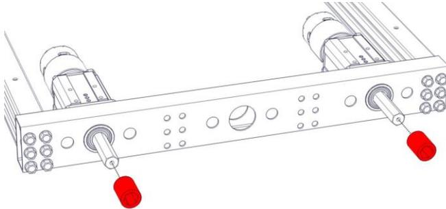
**Step 5:** Place one of each completed wheel assembly (left and right) onto the two drive shafts. The hub flange should be to the outside of the assembly. The roller axes at the top of the wheels should point towards the middle of the chassis.
