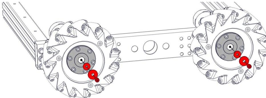
**Step 7:** Repeat Steps 1-6 to build the other half of the chassis. Be sure to mirror the assembly left-to-right and orient the Rover Side Rail such that the 24 End Rail holes are in the same vertical orientation as the previous assembly. The wheels should be put on the same way so that the rollers form an X on top (diamond on bottom).
