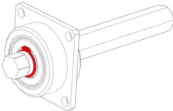
**Step 2:** The short output shaft needs to be replaced with the longer 3 inch output shaft. Using a pair of snap ring pliers, remove the snap ring from the backside of the face plate. Be careful not to permanently deform the snap ring by opening it too wide.
