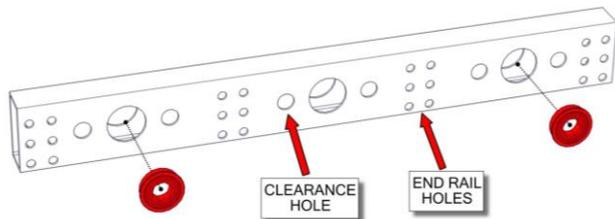
**Step 2:** Insert four (4) #10-32 x 0.625 inch Socket Head Cap Screws (am-1007) through the clearance holes and use four (4) #10-32 Nylock Jam Nuts (am-1063) to attach two gearbox assemblies to the tube. Align the hex bearings with the output shafts to allow them to slide through.
