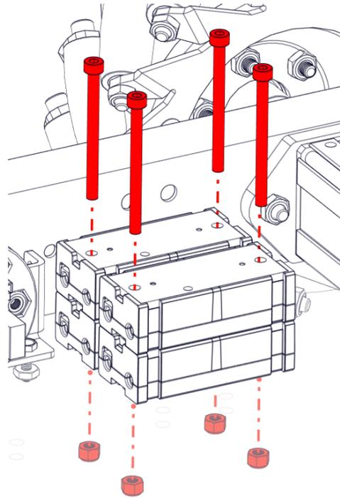
**Step 6:** Attach the 120A Circuit Breaker (am-0282) on the other side of the robot from the previous components using two (2) ¼-20 x 1.0 inch long Socket Head Cap Screws (am-1341) and ¼-20 Nylock Nuts (am-1015) on the underside of the Bottom Plate.
