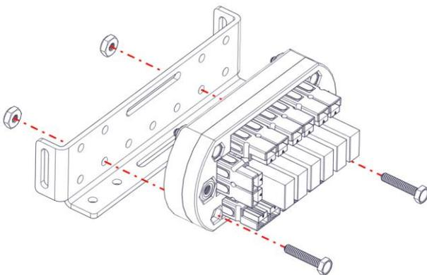
**Step 3:** Mount the PowerPole Distribution Board assembly to the top of the Bottom Plate using four (2) 0.5IN 6-32 Socket Head Cap Screws (am-1563) and 6-32 Nylock Nuts (am-1419) on the underside of the Bottom Plate.
