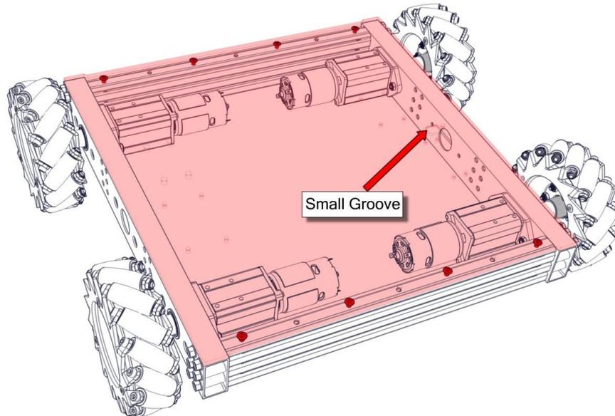
**Step 9:** The six (6) remaining holes along the End Rails should align with the through-holes in the End Rails but may need to be drilled out using a 1/4 inch bit to ensure a bolt may pass through.
