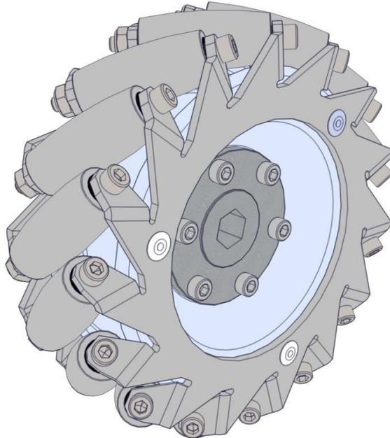
**Step 1:** Using six (6) #10-32 x 0.750 inch Socket Head Cap Screws (am-1047) and six (6) #10-32 Nylock Jam Nuts (am-1063), attach a ½ Inch Hex Hub (am-2568) to the wheel. The hub will protrude partially through the center of the wheel.
