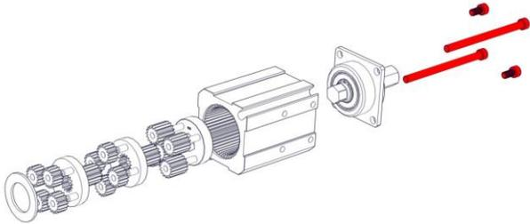
**Step 3:** Remove the output shaft by pulling it through the front of the face plate and bearings.
