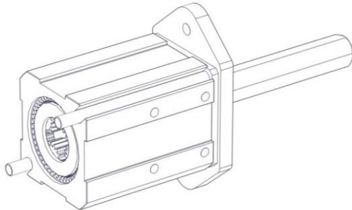
**Step 9:** Join the 57 Sport Gearbox and the motor together using the #10-32 x 3.0 inch Socket Head Cap Screws. Make sure the thrust washer is seated in the ring gear flush against the planet gears before mating the two housings.
